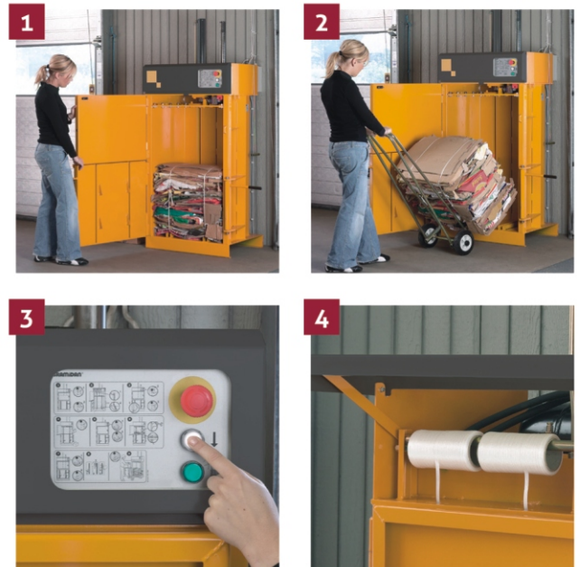
1 Compact your waste and eject the finished bale. 2 Remove and store the bale until collection. 3 The baler has a simple control panel and is equipped with easily understood pictograms. 4 The strap rolls are easy to replace in front of the machine.
