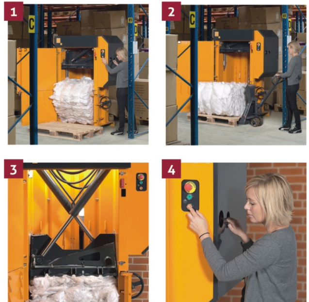
1 Compact your waste and eject the finished bale. 2 Remove and store the bale until collection. 3 The cross cylinders ensure stable compression and a low overall height. 4 The bale is ejected by a safe two-hand operation.
